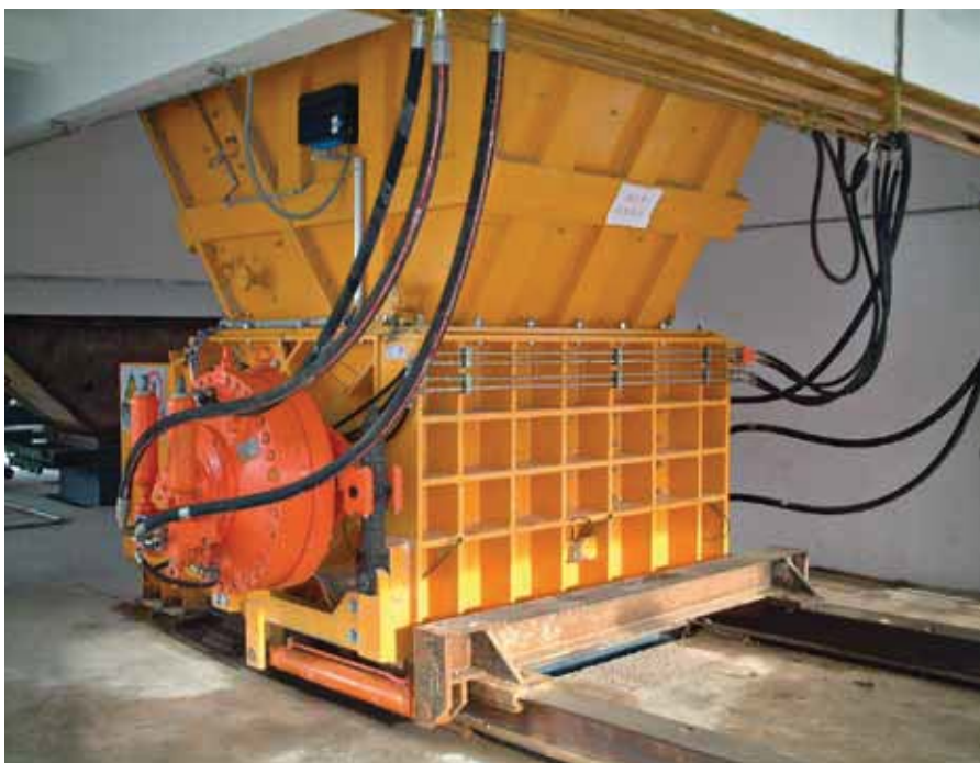
1 Robust shredder for opening, dissolving and homogenization
